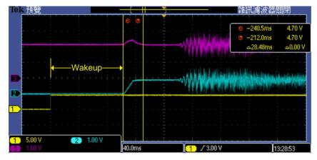
Input signals in the interval of Wakeup time. The front voice signals during Wakeup time are truncated.
